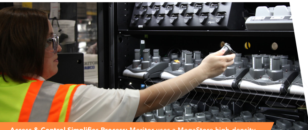
Access & Control Simplifies Process: Meritor uses a MegaStore high-density dispensing system to store and charge handheld batteries.
